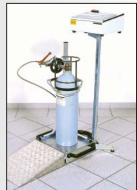
Fig. 3: Digital floor scales for CO 2 bottles 2 – 20 kg, with programmable display unit and automatic cut-out, including drop-down ramp (without bottle).
