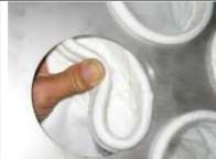
Shake to Clean Filter. If necessary, Remove and replace
